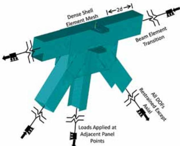
Figure 3. Example of finite element model and boundary conditions for truss bridge joints.
