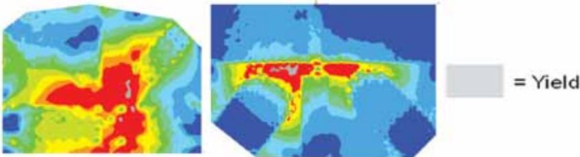
Figure 4. Stress contours (Von Mises stress) in the gusset plates for two of three joints at the onset of gusset plate yielding.
