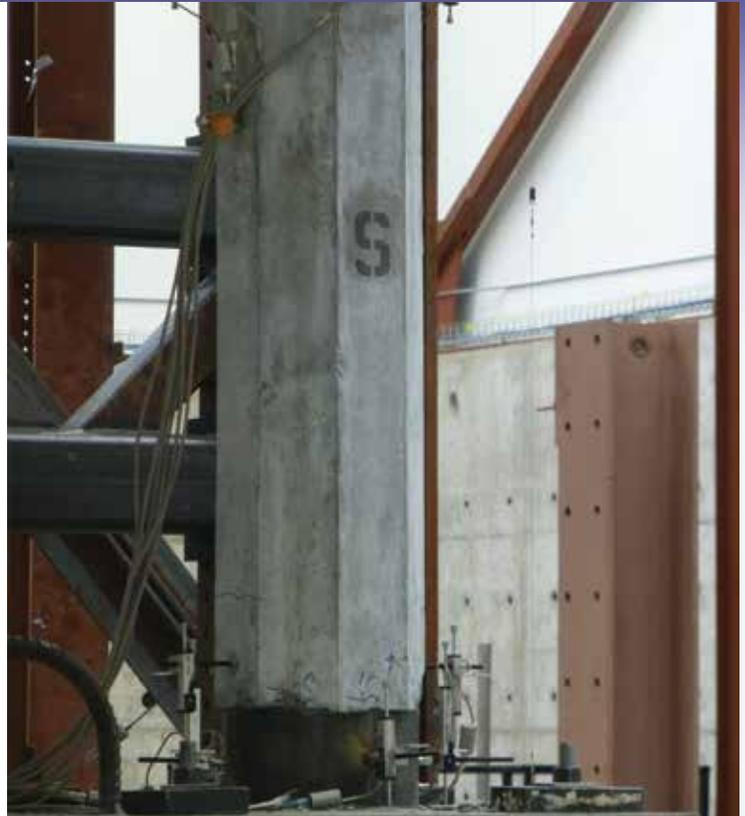
*One of the bridge columns at the end of all the shaking table tests.*
