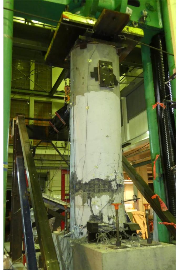
**Pile-column under test**
