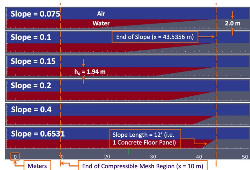
**Simulation of Structure in Flume**
