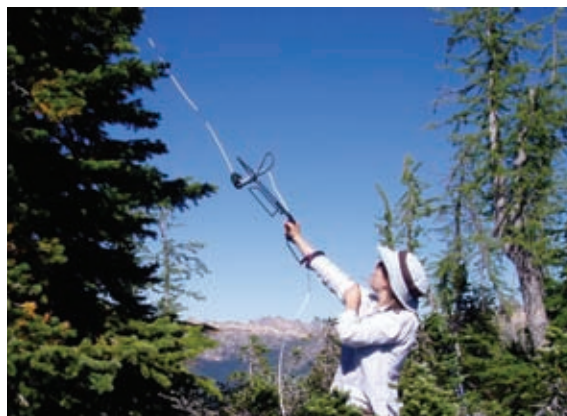
Jessica Lundquist, assistant professor, launches a self-recording temperature sensor into a tree in the North Cascades to test how temperature varies across the landscape and how temperature patterns match with snow duration, measured by temperature sensors on the ground.
