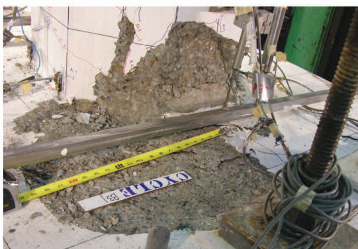
Damage at the end of pile testing of the CR connection.
