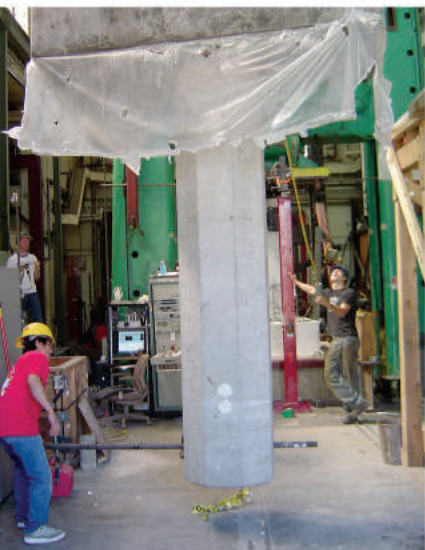
Placing a full-scale pile-to-wharf connection for structural testing.
