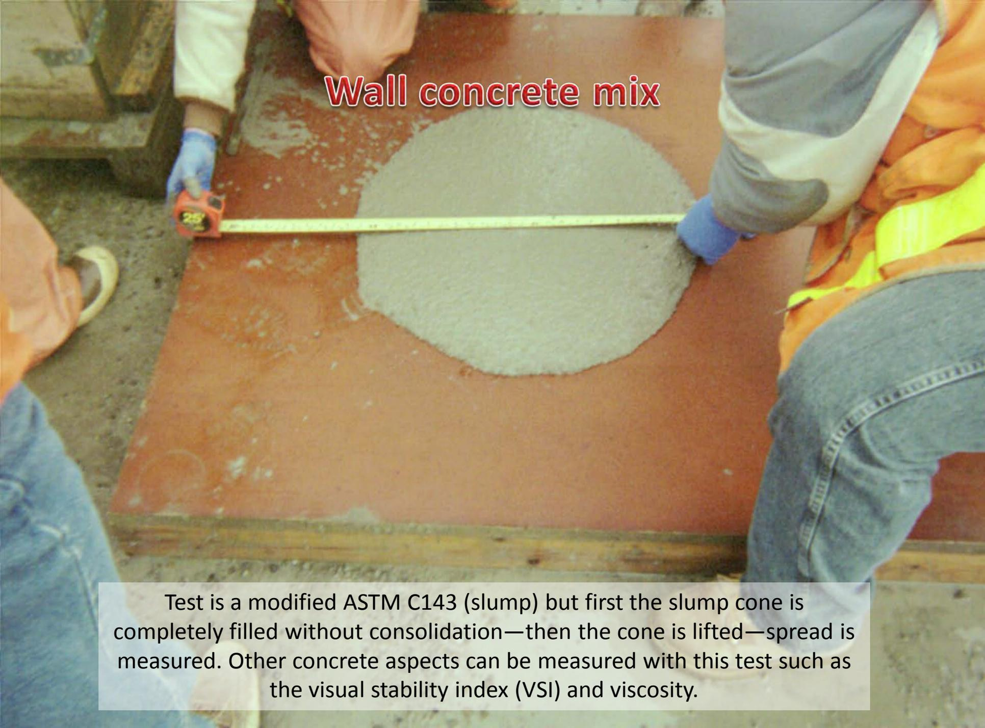
Test is a modified ASTM C143 (slump) but first the slump cone is completely filled without consolidation—then the cone is lifted—spread is measured. Other concrete aspects can be measured with this test such as the visual stability index (VSI) and viscosity.
