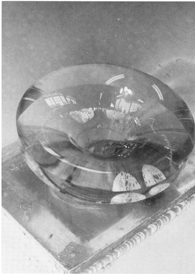
Figure 4. Spillway, No Piers, Rooster-Tail on Dam Axis Side
