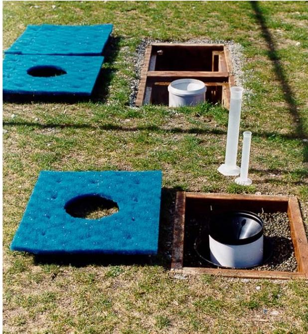
**Figure 4-4:** The buried TB3 tipping-bucket trench gauge (top) and the buried Novalynx gauge (bottom)
