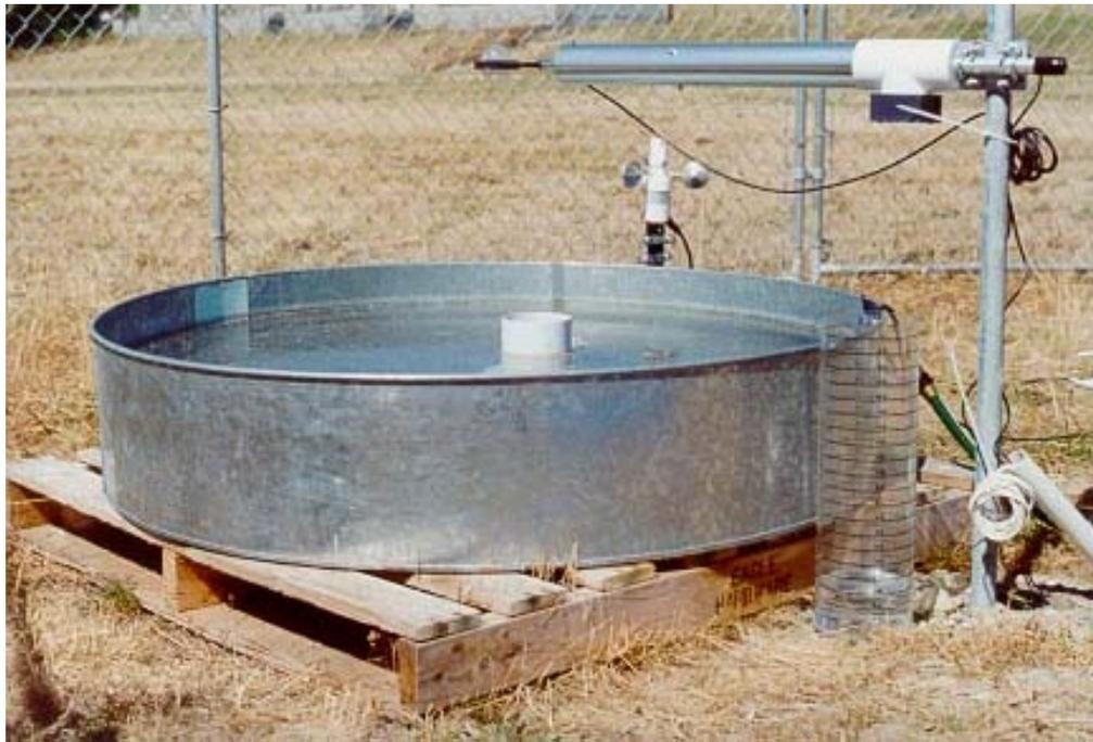
**Figure 4-3:** The evaporation pan collection system
