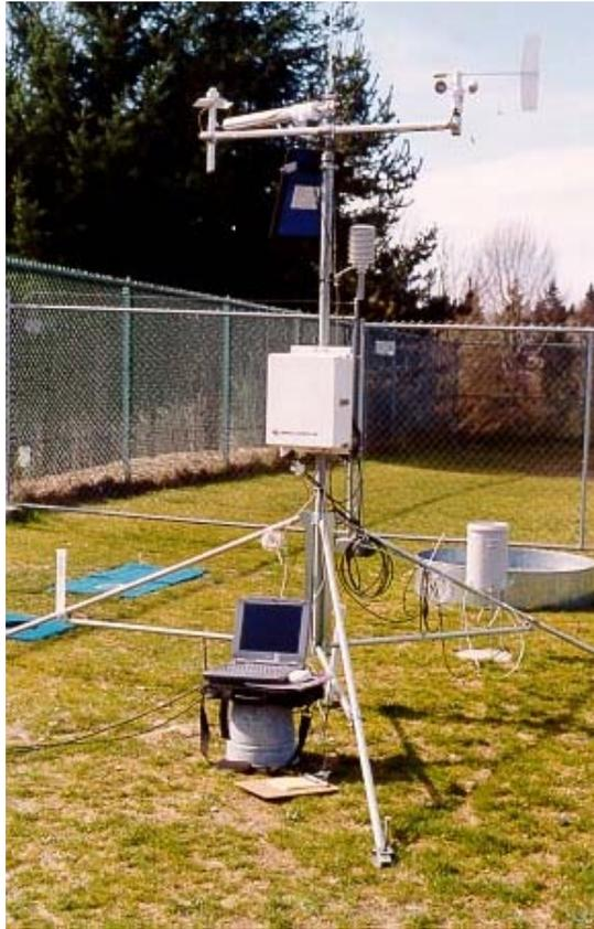
**Figure 4-1:** The CM10 Tripod Weather Station located at the Viewlands swale monitoring station
