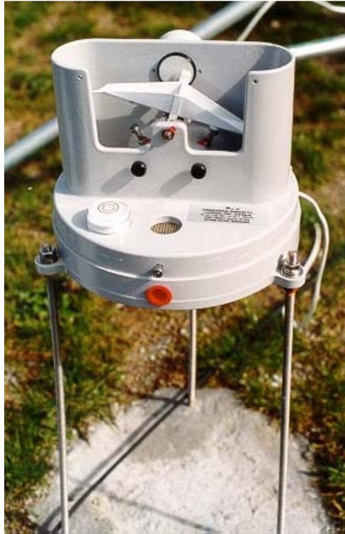
**Figure 4-5:** The standing TB3 tipping bucket gauge
