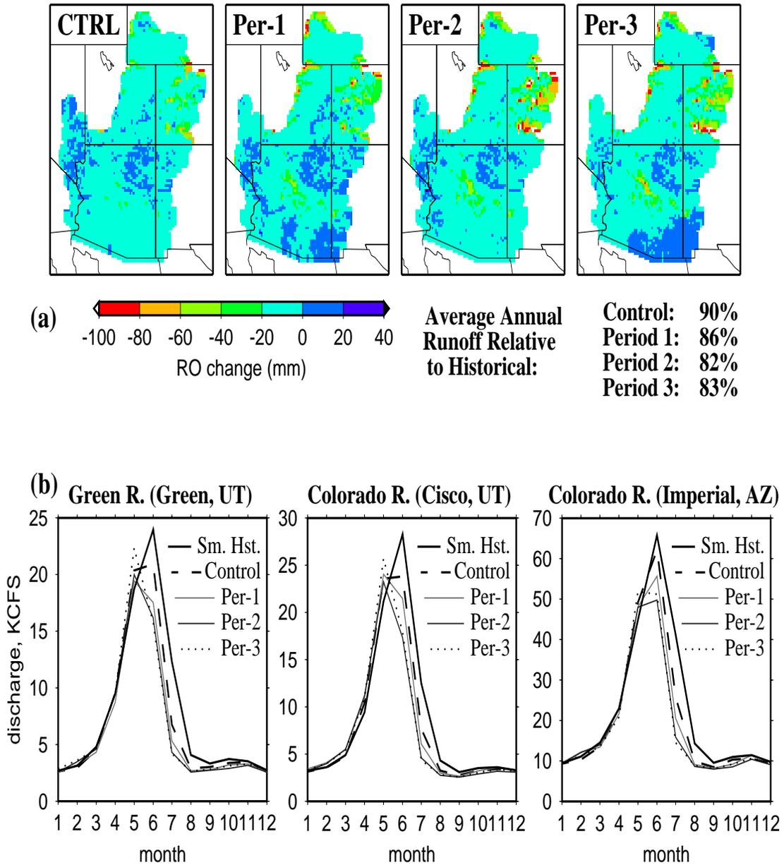
**Figure 8** (a) Spatial distribution of predicted changes in mean annual runoff for control and BAU Periods 1-3 (averaged over 3 ensembles) relative to historic, and (b) mean monthly hydrograph for the Green River at Green River, UT, Colorado River near Cisco, UT, and the Colorado River below Imperial, AZ for historic, control, and BAU period 1-3 simulations (BAU results averaged over 3 ensembles).
