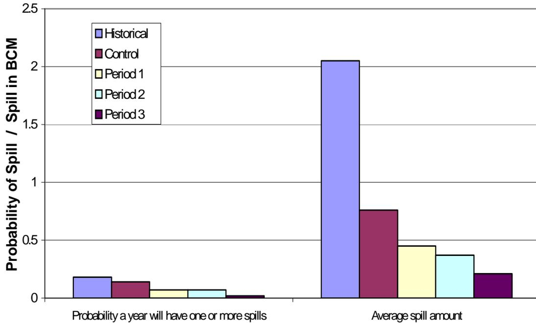
**Figure 14** Probability a given year will have an uncontrolled spill (release that does not generate hydropower) and average amount of spill for historical, control, and BAU Period 1-3 simulations (BAU results averaged over 3 ensembles).
