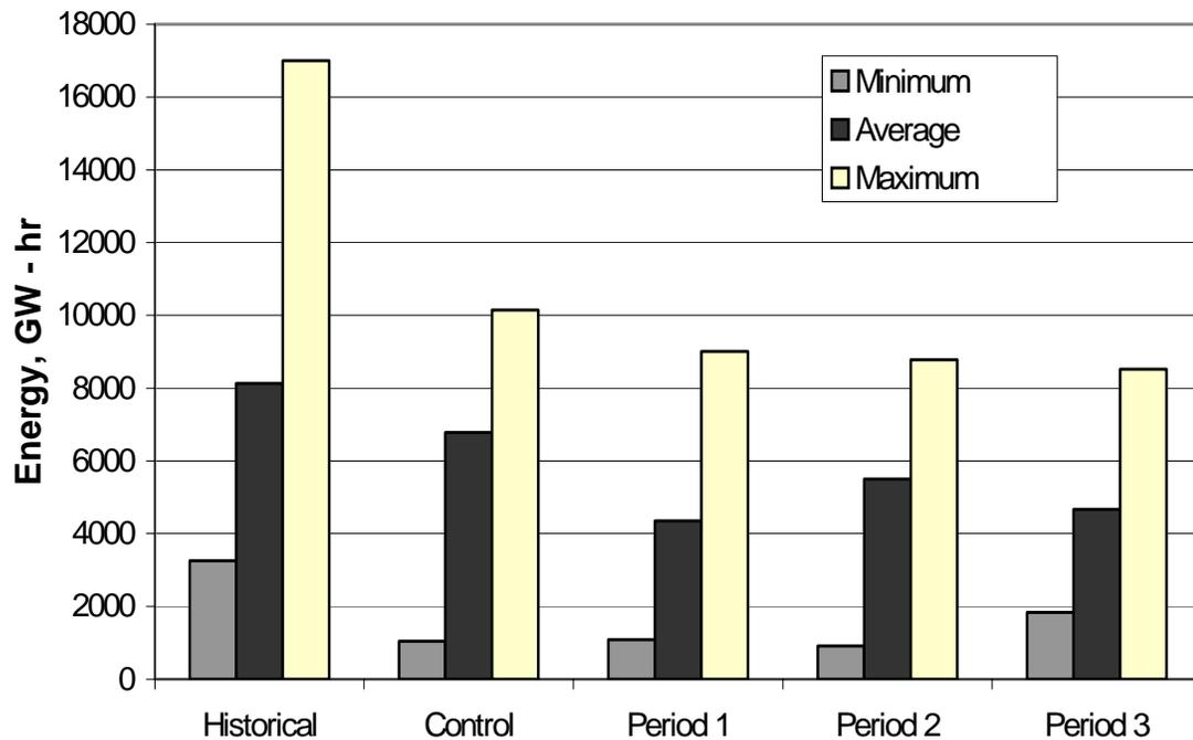
**Figure 13** Simulated minimum, average, and maximum total basin energy production for historical, control, and BAU Period 1-3 simulations (BAU results averaged over 3 ensembles)
