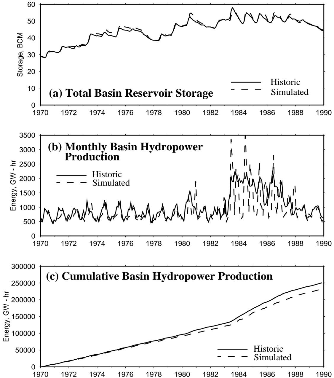
**Figure 5** (a) CRRM simulated and observed total basin storage for 1970-90; (b) CRRM simulated and observed total basin monthly hydropower production for 1970-90; (c) CRRM simulated and observed cumulative hydropower production for 1970-1990.
