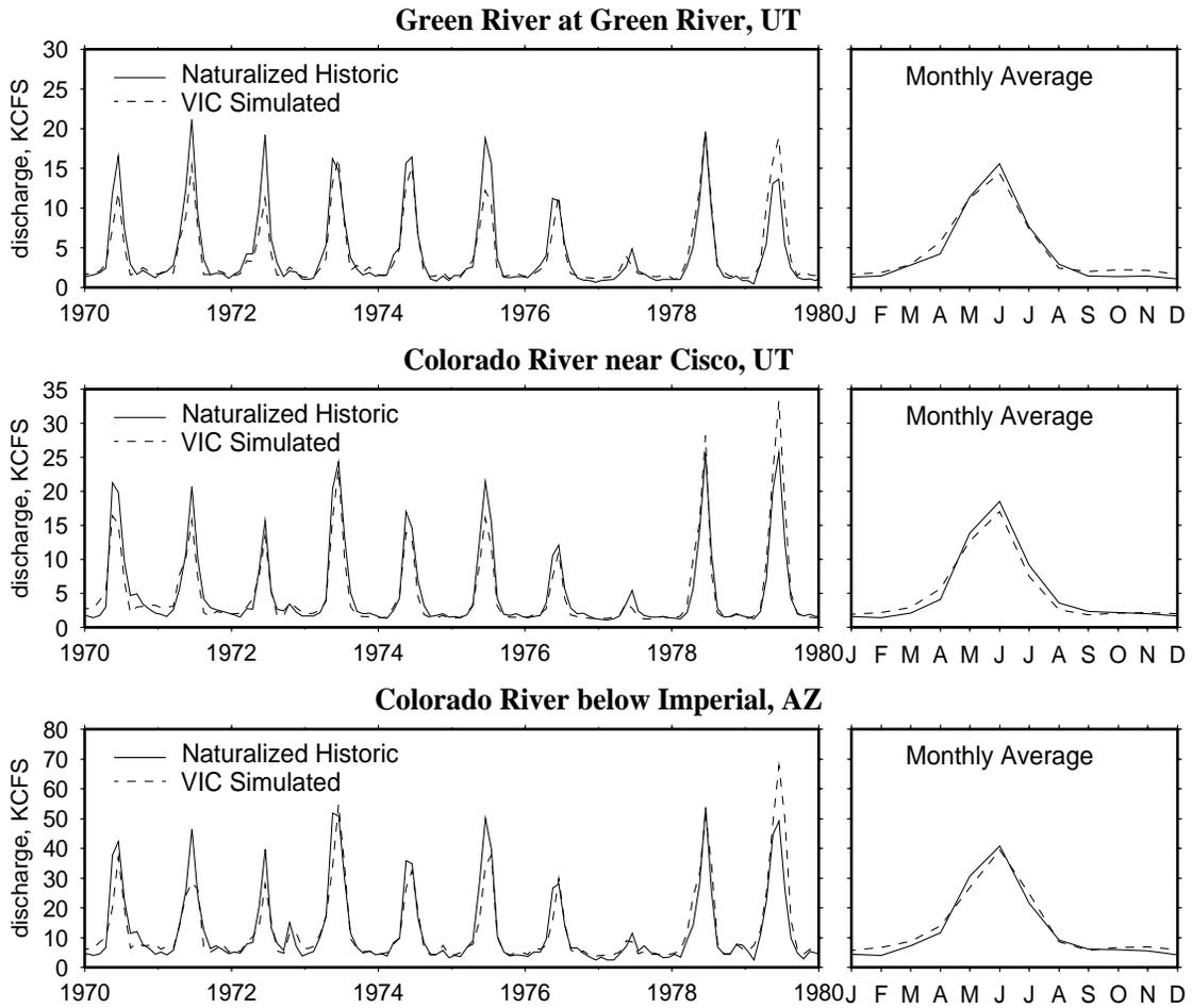
**Figure 4** VIC simulated and naturalized historic observed streamflows at Green River, UT, Cisco, UT, and Imperial, AZ for 1970-1980.
