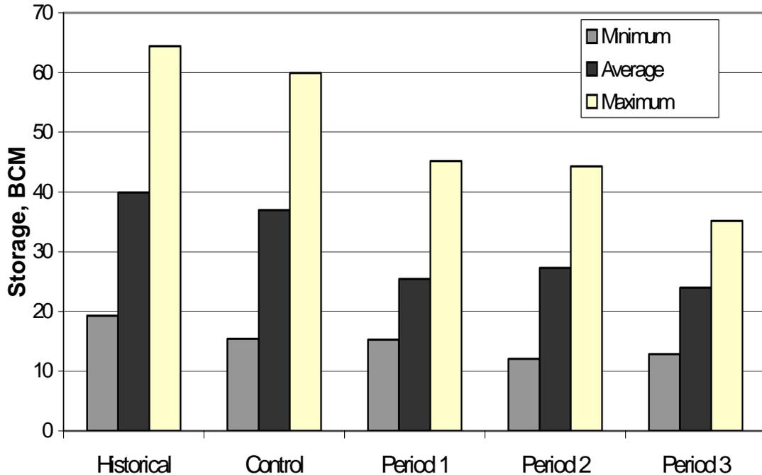
**Figure 9** Simulated minimum, average, and maximum total basin storage for historical, control, and BAU Period 1-3 simulations (BAU results averaged over 3 ensembles).
