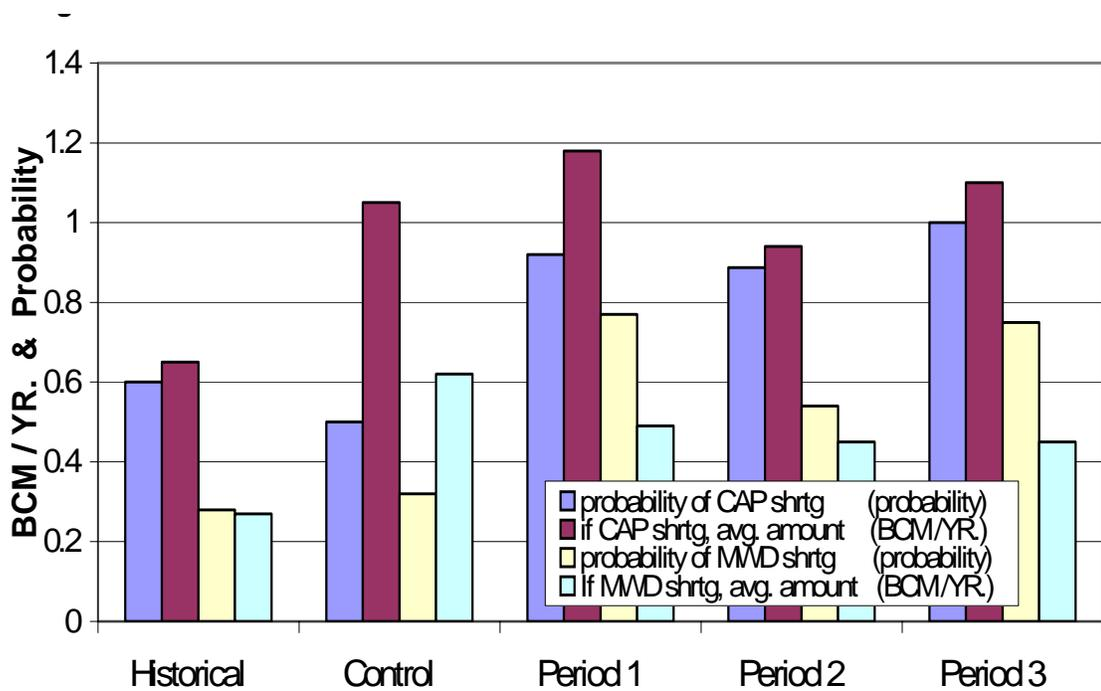
**Figure 12** Probability of a delivery shortage to CAP and MWD and average amount of shortfall for historical, control, and BAU Period 1-3 simulations (BAU results averaged over 3 ensembles).
