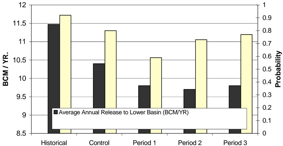
**Figure 10** Simulated average annual release from Glen Canyon Dam to the lower basin and probability that release targets are met for historical, control, and BAU Period 1-3 simulations (BAU results averaged over 3 ensembles).
