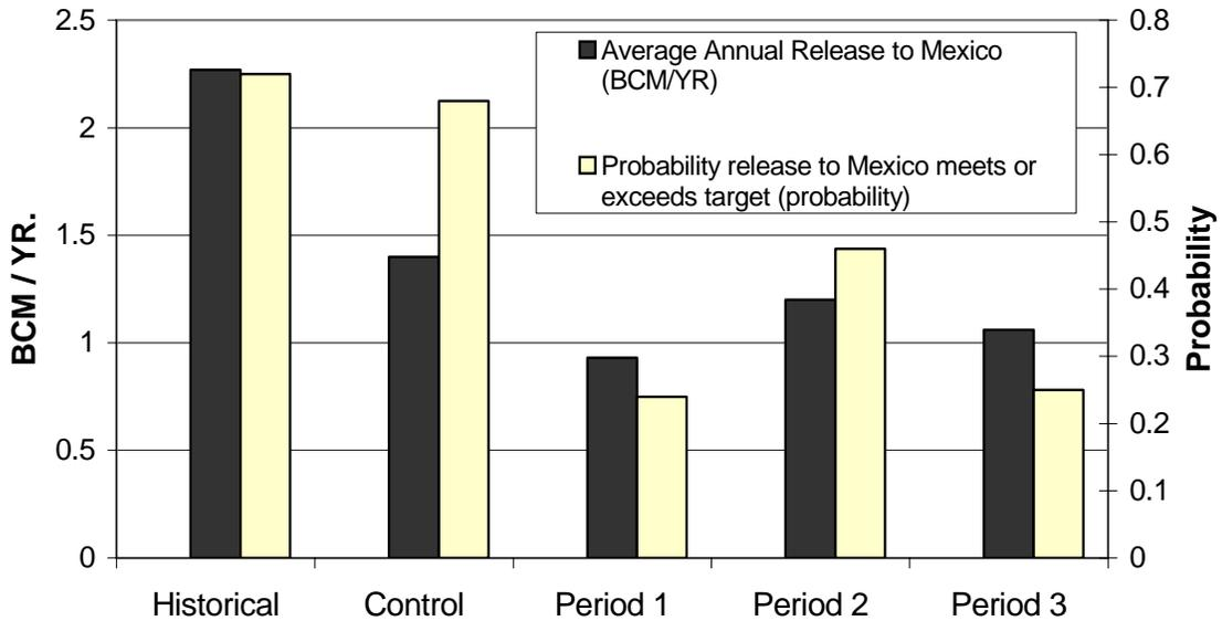
**Figure 11** Simulated average annual release from Imperial Dam to Mexico and probability that release targets are met for historical, control, and BAU Period 1-3 simulations (BAU results averaged over 3 ensembles).
