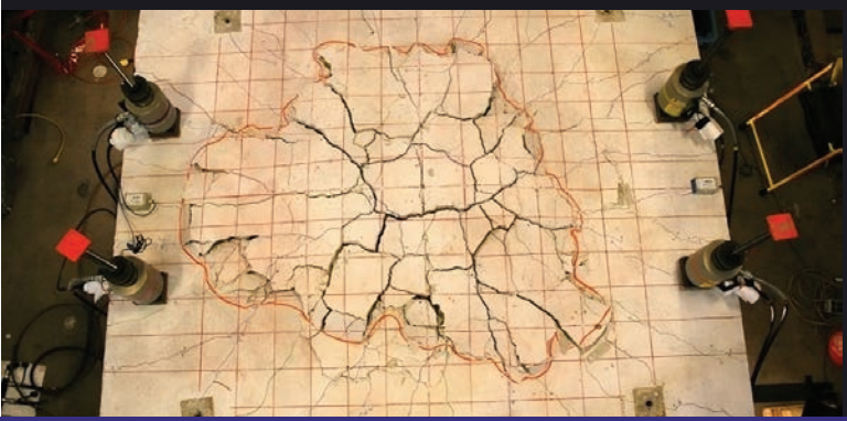
Top view of a slab after a punching shear test, showing cracks radiating outward from the center, where the column supported the slab from below. Photo courtesy of NIST.
