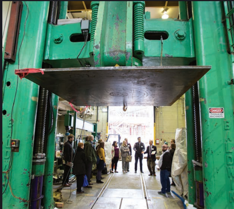
CEE’s 2.4 million pound Universal Testing Machine in the Large-Scale Structural Engineering Testing Lab was used to test columns during the investigation.
