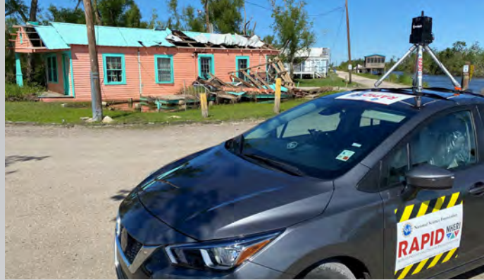
Following Hurricane Ida, RAPID researchers collect data throughout Grand Isle, Louisiana, using a 360-degree Street View camera system mounted on top of a vehicle.
