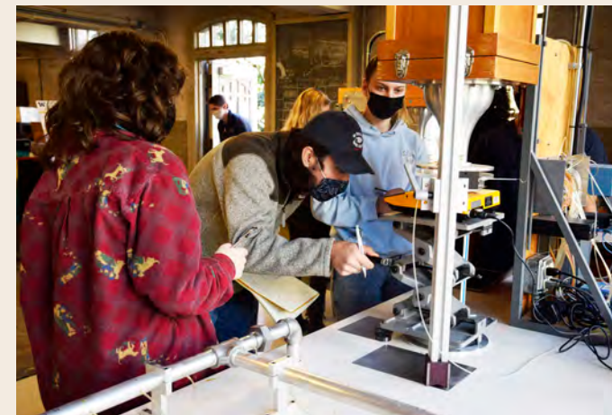
During an introduction to fluid mechanics (CEE 347) lab where students learn to measure the force of an air jet, junior Ingrid Phillips (left) watches junior Daniel Tsukada (center) adjust the height of the force scale. The students are gathered around one of three air flow benches relocated to the renovated lab space.
